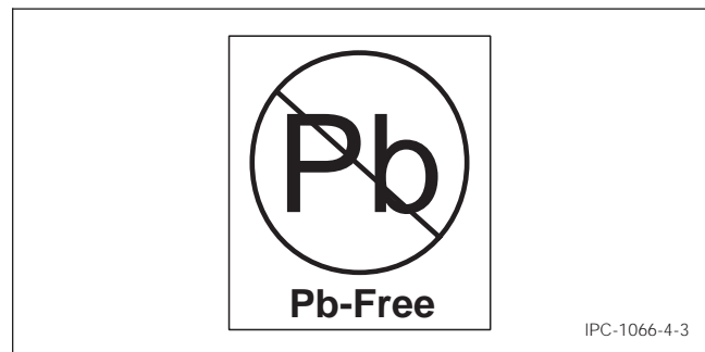
Figure 4-3 Pb-Free Identification Label
